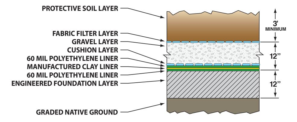
The MRL liner design exceeds the Federal and State standards. Both require a single 60 mil liner over a clay liner.
